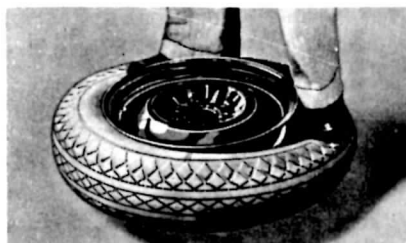
DISLODGING CASING FROM RIM
